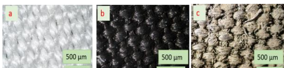
Figure 1: Optical microscopy image of a) cotton, b) PPy-cotton and c) Silver coated PPy-cotton.
